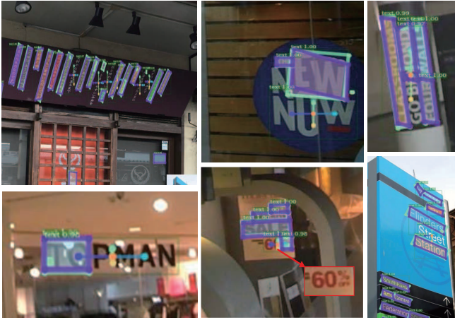
Figure 5: Examples that SBD can recall many instances that segmentation branch fails to recall. Green bounding boxes and scores represent RoIs. Rotated cyan bounding box and transparent pixels represent the result from segmentation branch. Transparent pixels are predicted by mask branch. Purple quadrangles are final detection results from SBD. KEs are simplify by colorful points.
