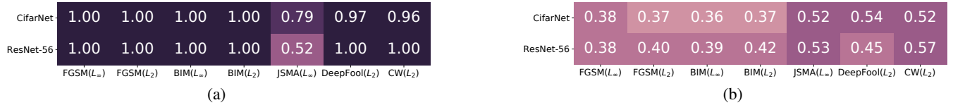
Figure 5: Black-box detection against transferred attacks across different classifier models: (a) Ours and (b) Feature Squeezing. Our detector was trained with FGSM ( l_\infty ) on ResNet-20 and tested by another attack (column) built on two substitute models, namely CifarNet (upper row) and ResNet-56 (lower row) over CIFAR-10.
