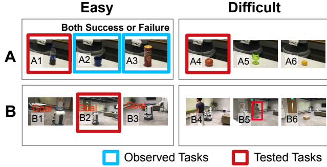
Figure 1: Trust Transfer Experiment Design (Household domain). Each row represents a task category: (A) picking and placing objects, and (B) navigation in a room. Tasks were further categorized into Easy and Difficult tasks. See text for more details.
