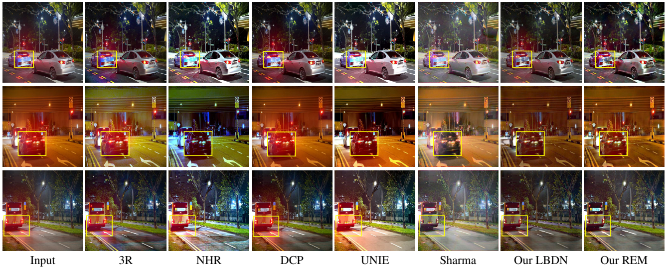
Figure 7: Some examples of visual comparisons on the light-effects dataset [Sharma and Tan, 2021]. Our LBDN achieves the most visually significant glow suppression, and REM further reinforces the visibility with appropriate luminance adjustments.
