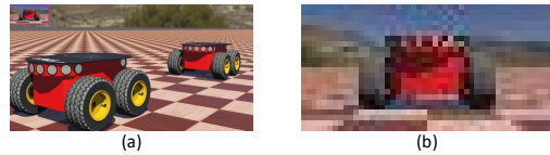
Figure 5: (a) Simulated ACC in Webots: The ego car (left) follows the reference car (right); (b) An example camera image.
