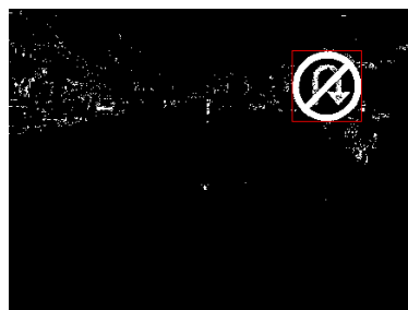
Fig. 5. An example of traffic sign detected by color segmentation.
