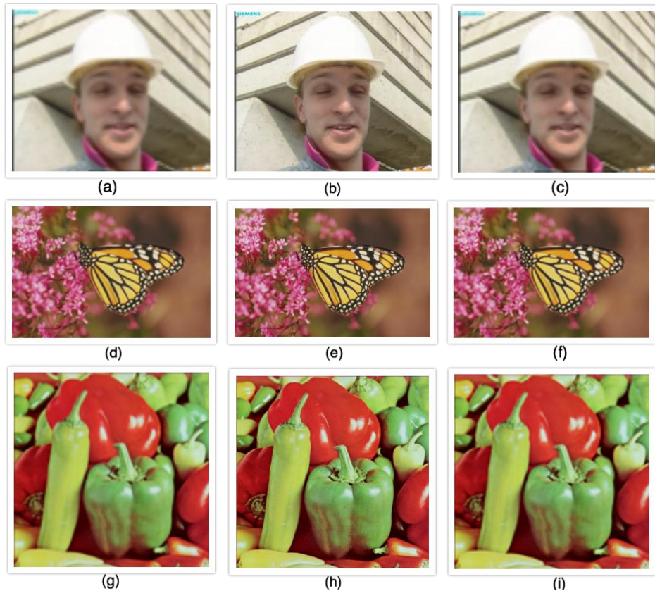
Fig. 6. Visual Comparison between LR images - (a),(d),(e), ground truth HR images - (b), (e), (h) and reconstructed images - (c), (f), (i) at scale 4
