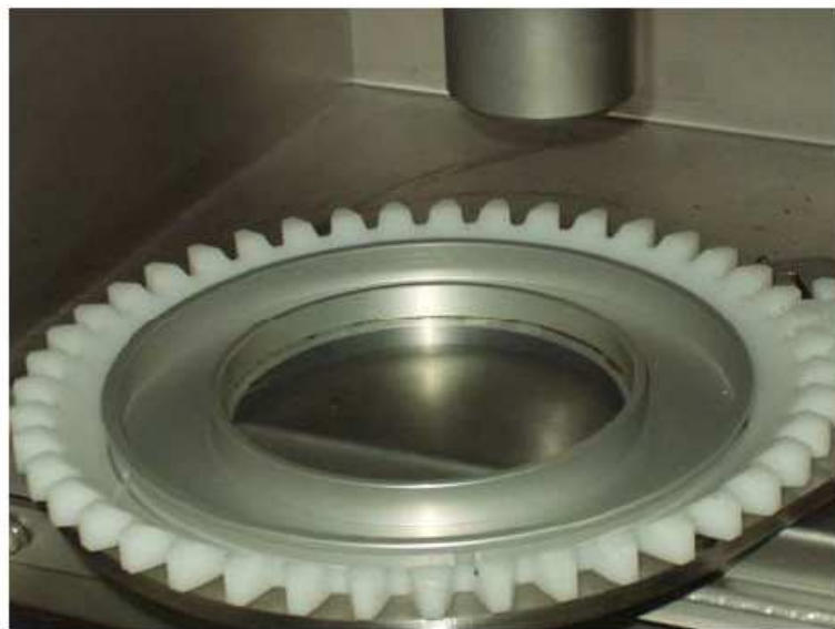
Crown gear permitting measurement of different areas of the sample
