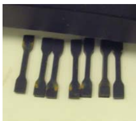
Figure 3 –The specimens moulded by Type 4 – ASTM D638-03
