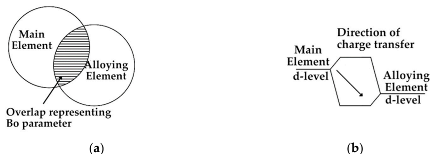
Figure 1. Graphical representation of Bo (a) and Md (b) parameters.
