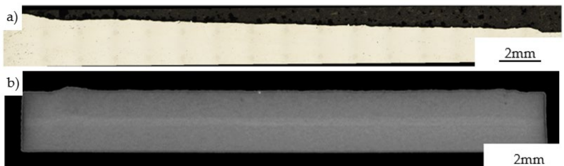
Figure 6. Microstructure of the longitudinal section with optimization of the application parameters (heated substrate, three layers across the thickness) (a); tomographic longitudinal section of the final cladding (b).
