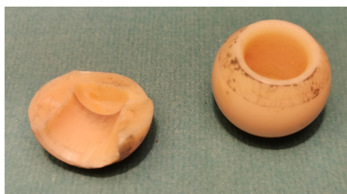
Figure 2. Fragmentation (break) of ceramic head of the hip prosthesis that succumbed to accidental overload with mechanical forces of high amplitude.
