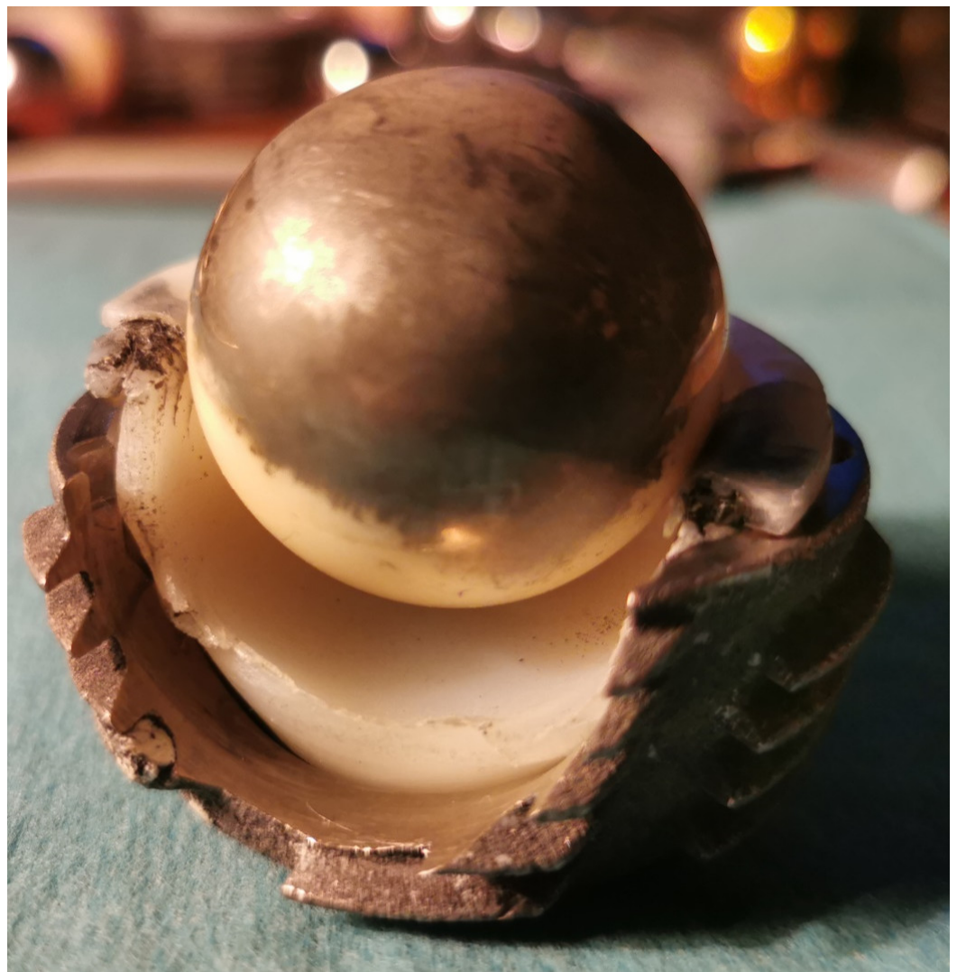
Figure 5. An example of the acetabular cup grinding and its UHMWPE insert by Al 2 O 3 ceramic head during decades-long weight bearing.
