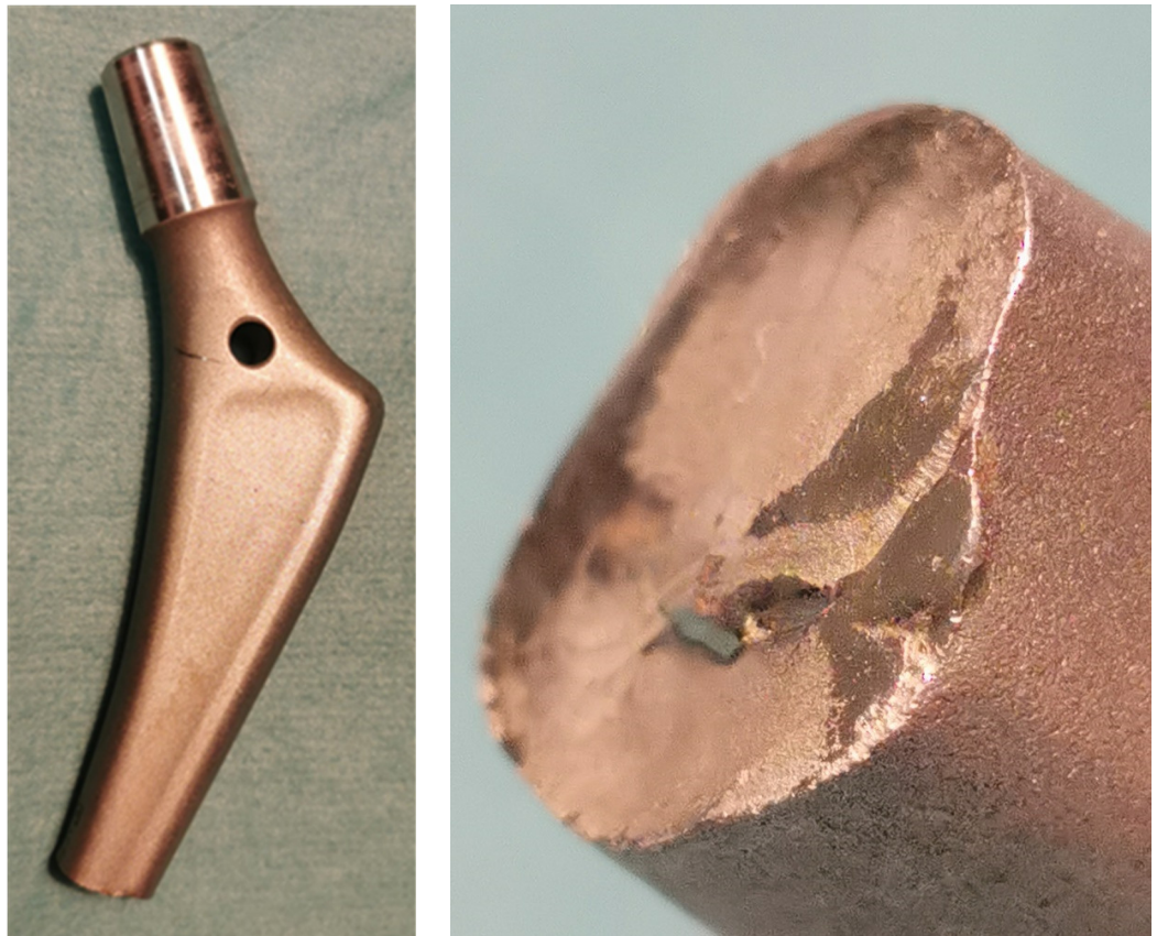
Figure 6. Break of the stem of the hip prosthesis and macro-photograph of the surface of its break-through.
