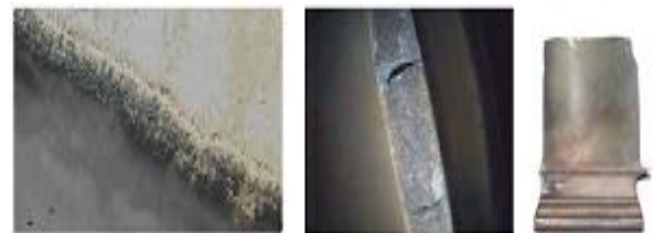
Fig 2.6: Characteristic forms of failures caused by overheating of blade material
