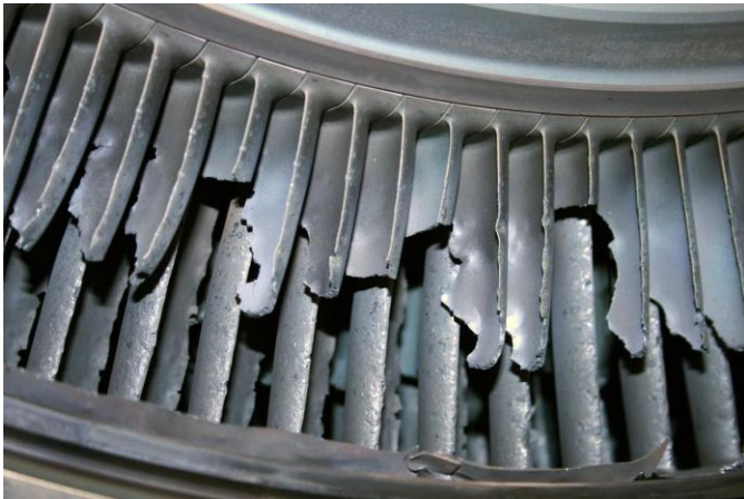
Fig 2.3: blade failure due to overheating
