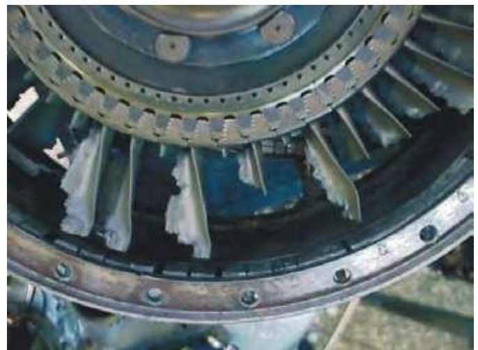
Fig 2.7: Characteristic forms of failures to gas turbine caused by long-lasting excessive temperature of exhaust gases
