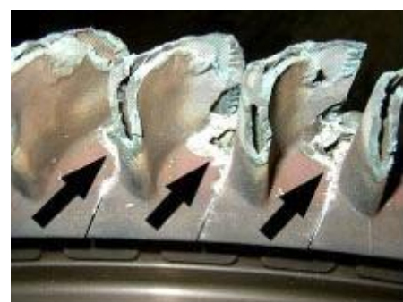
Fig 2.2: blade failure due to fatigue
