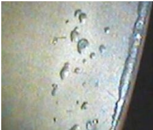
Fig 2.8: Failures to turbine blades operated in the seashore environment, caused by chemical impact of exhaust gases
