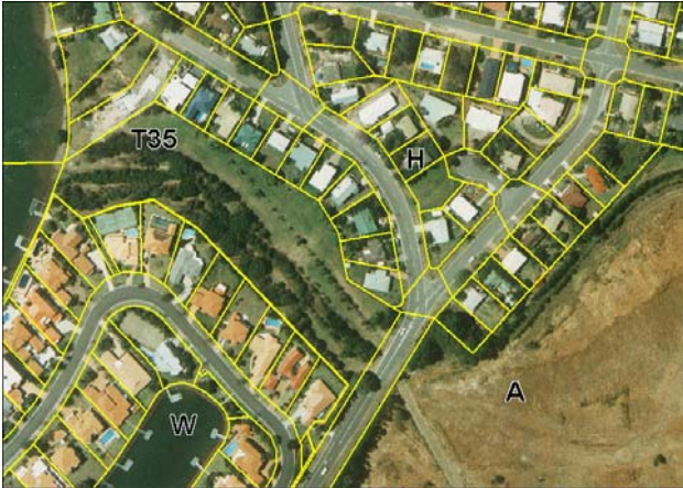
Figure 4. Parcel-based classification of land cover including the percentage of tree cover. ‘A’ denotes ‘Agriculture’, ‘H’ – ‘House’, ‘T35’ – 35% of ‘tree’ cover, and ‘W’ – ‘water’.
