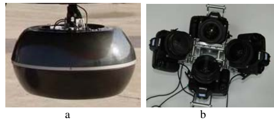
Figure6. a, b the appearance and inside of super-wide-angle camera
