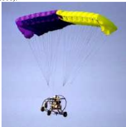
Fig. 5 Powered paraglider (Thamm, 2006)
