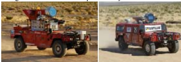
Figure 3: Sandstorm (left) and Highlander (right) were developed to navigate at high-speed in desert terrain.
