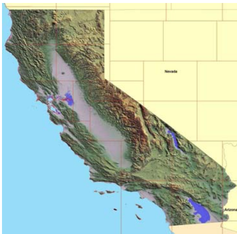
Figure 3. NEXTMAP USA Example - California DSM, validated vertical accuracy (1430 check points) 0.76 m RMSE
