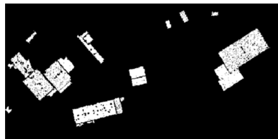
Fig.7. Building segment by area threshold
