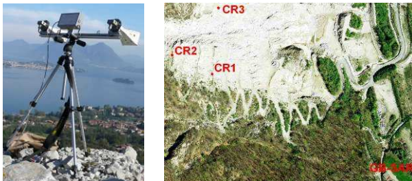
Figure 5. Active radar calibrator (left) and the CR1, CR2, CR3 positions in which it has been installed (right) in order to correctly locate the acquired SAR images
