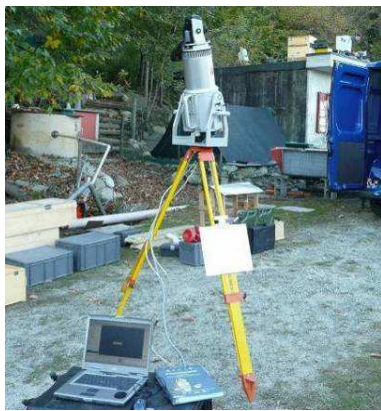
Figure 8. The Riegl LMS-Z420 Laser scanner
