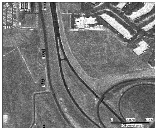
(b). High resolution image from Star3i system (135 MHz bandwidth)
