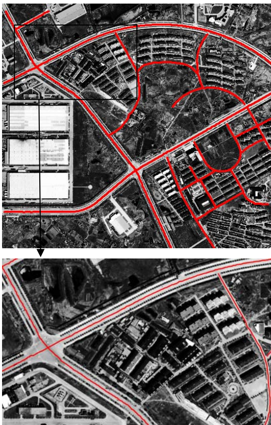
Fig. 4 Semi-automatic extracted road network on Quickbird image (a) Overview (b) Local result.
