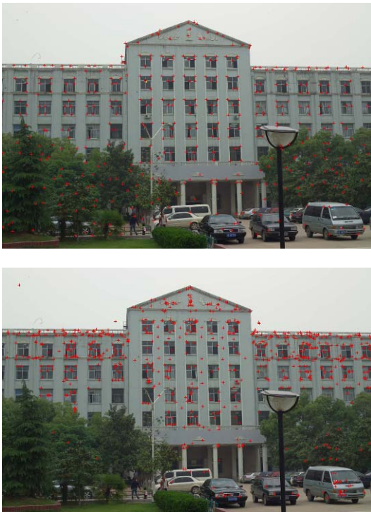
Figure.2 Distinct points extracted by Harris (top) and SIFT (bottom).
