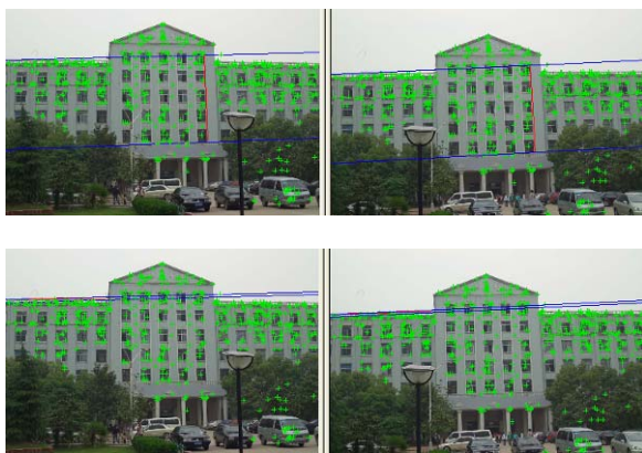
Figure.5 Top row pictures show the epipolar line constraint for a vertical line, while bottom row pictures show this constraint for a horizontal line. In four pictures, red lines represent extracted feature lines and blue lines represent epipolar lines.
