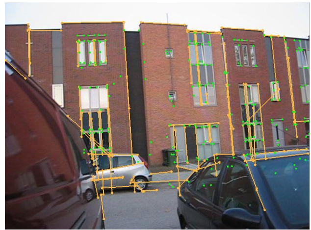
Figure 2. Input video image sequence with reliable points and extracted edges, Reliable points (green), edges with end points (yellow) frame 0 (upper), frame 133 (lower)
