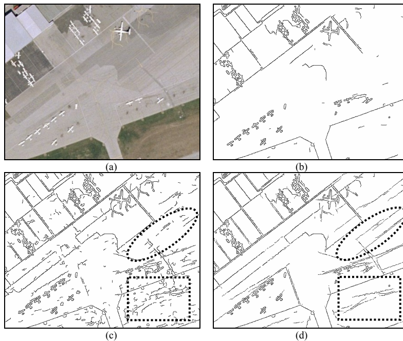
Figure 6. Results of the first experiment. (a) Input Image. (b) Result of Edison algorithm with tight thresholds. (c) Result of Edison algorithm with loose thresholds. (d) Result of the proposed algorithm.
