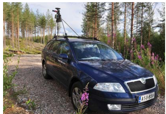
Figure 4: The MMS system mounted on car
