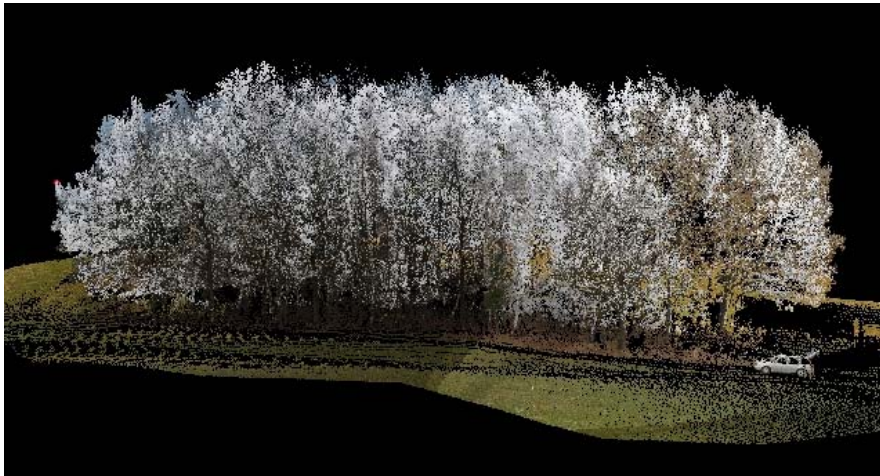
Figure 1. TLS point cloud of reference grove '08_Reg_hohFg'
