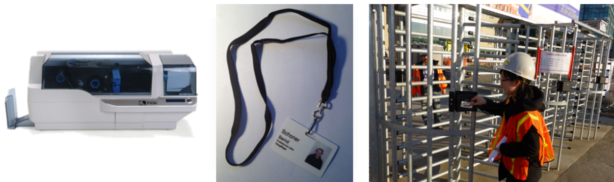
FIG. 2: Hardware components: RFID badge printer (left); passive RFID badge (center); and RFID turnstile (right).
