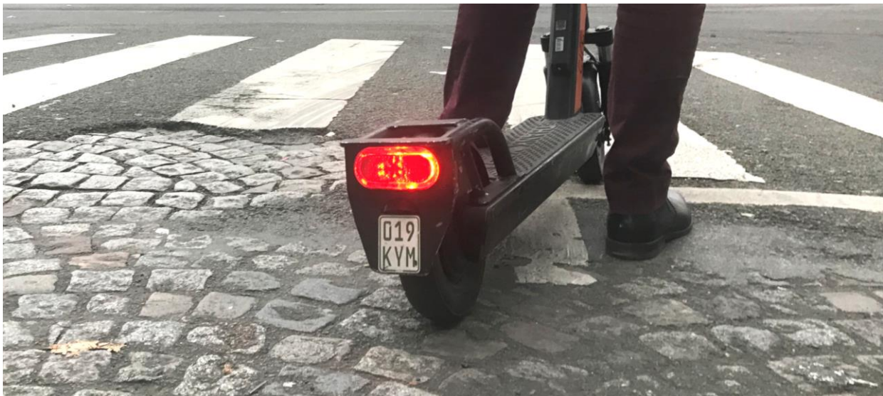
Figure 17. E-scooter identification plate in Europe
