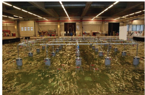
Figure 4 WEC array with 25 heaving buoys from the WECwakes project (taken from Troch et al., 2014)
