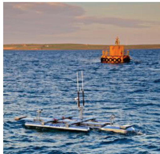
Figure 12 1/10th scale Magallanes test turbine installation at EMEC (EMEC, 2017)
