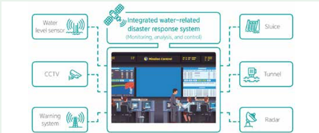
Figure 11. Integrated Water-Related Disaster Response System Source: K-water (2018) 20
