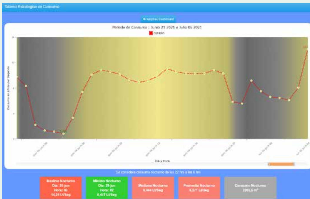
Figure 8. Hourly consumption of a specific account. In yellow, consumption during the day. In gray, nightly consumption. Useful for pressure control projects
