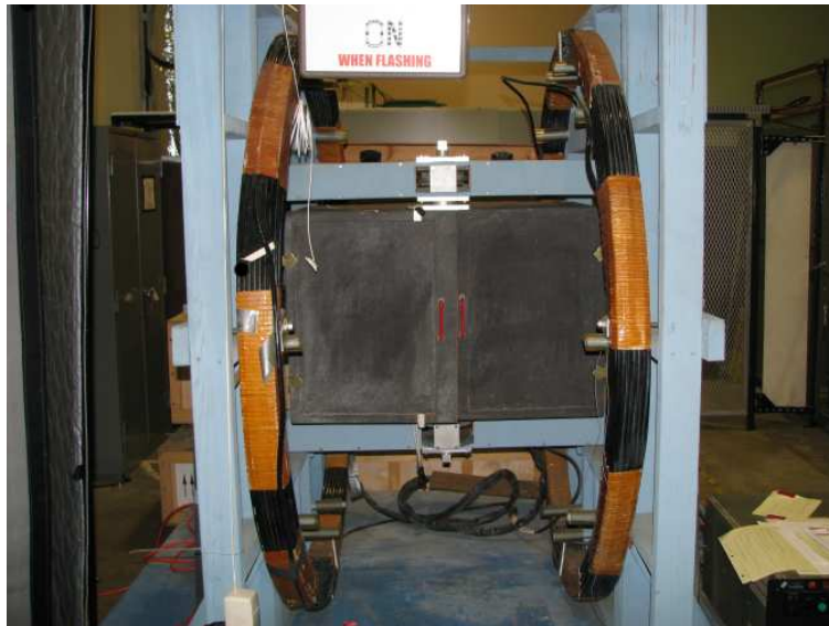
Figure 3.43: Photograph of the magnetic shielding test stand. The black box that contains the test shielding is located between the magnetic coils.
