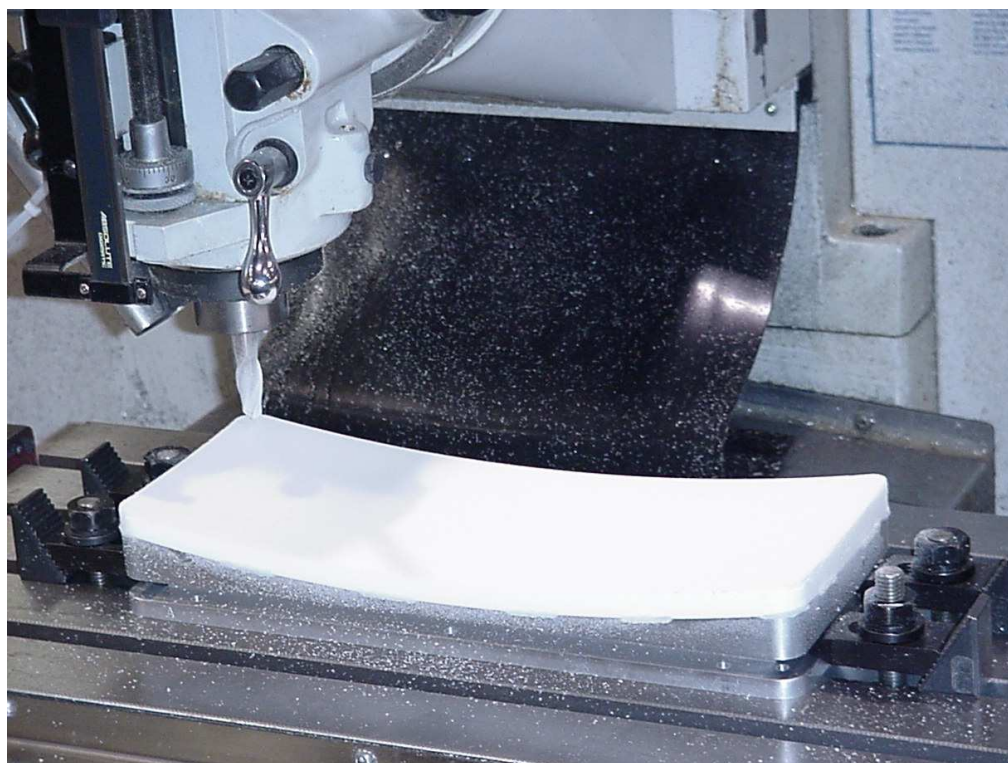
Figure 3.20: Computer-controlled cutting of the ellipsoidal surface of the foam substrate.
