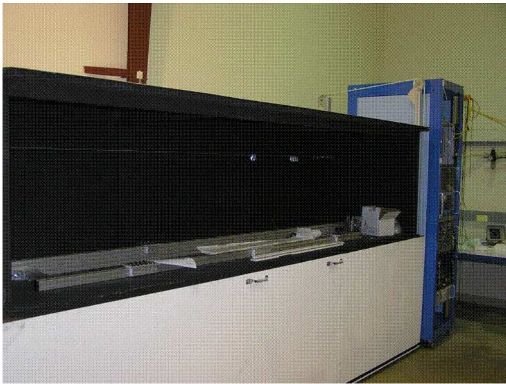
Figure 6.10: Picture of the dark box. The moveable cart is mounted on rails.
