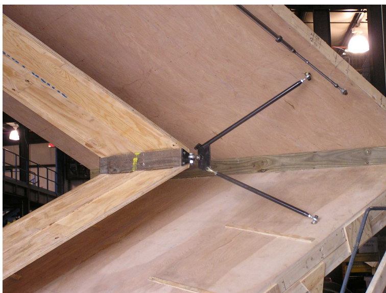
Figure 10.9: Photograph of the link system installed in the Region 2 drift chamber plywood prototype. The link systems for all 18 CLAS12 drift chambers will be of a similar design.
