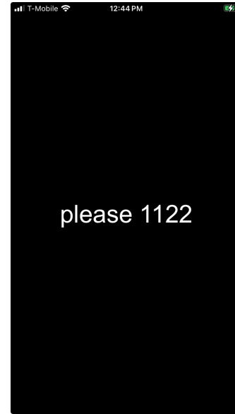
Figure 1: Example of the FlexType interface showing a user who is entering the phrase “please call”. The user has completely entered the word “please”, which is displayed in large high-contrast text. The user has selected the groups for each letter in “call”, but has not yet swiped right to perform recognition. The unrecognized taps are displayed using the selected group numbers “1122”.
