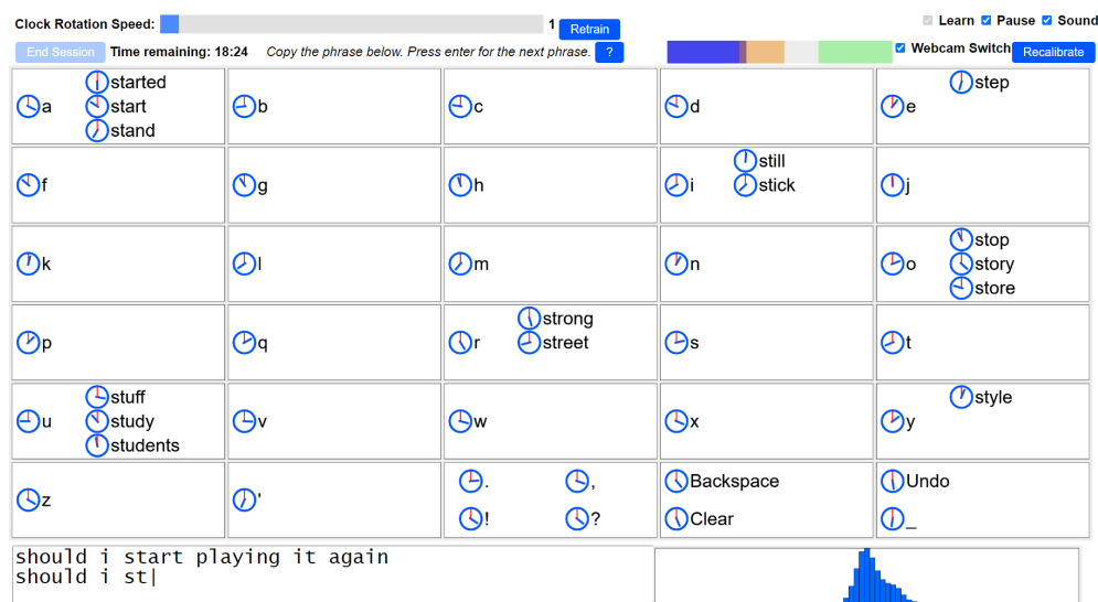
Figure 1: Nomon being used to enter the phrase “should i start playing it again”. The user has typed “should i st” thus far. To write the letter “a”, the user clicks a switch when the clock near “a” is at noon. Target selection may require multiple clicks depending on the user’s switch precision (visualized by the histogram). The user can select word completions to speed writing.
