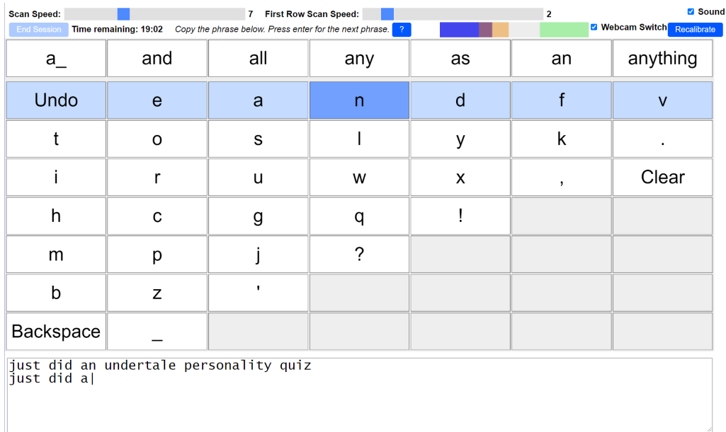
Figure 2: Our row-column scanning keyboard interface. The user is being prompted to write “just did an undertale personality quiz” and has written “just did a” so far. The interface progressively highlights rows until the user clicks their switch, and then progressively highlights columns within the selected row until the user clicks once more. Users can also select word completions that are displayed at the top.
