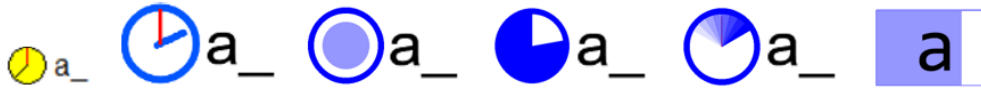
Figure 3: From left to right: (1) The clock used in the original Nomon interface [7], (2) the clock design used in this study, (3) the filling ball clock, (4) the “pac-man” clock, (5) the radar clock, (6) the progress bar. Clock sizes are relative to the clock from the original interface on a 2560 \times 1600 pixel display.
