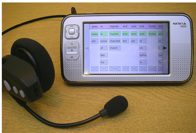
Figure 1. The Nokia N800 device and a Bluetooth headset. The Parakeet continuous speech recognition system is shown running on the device.
