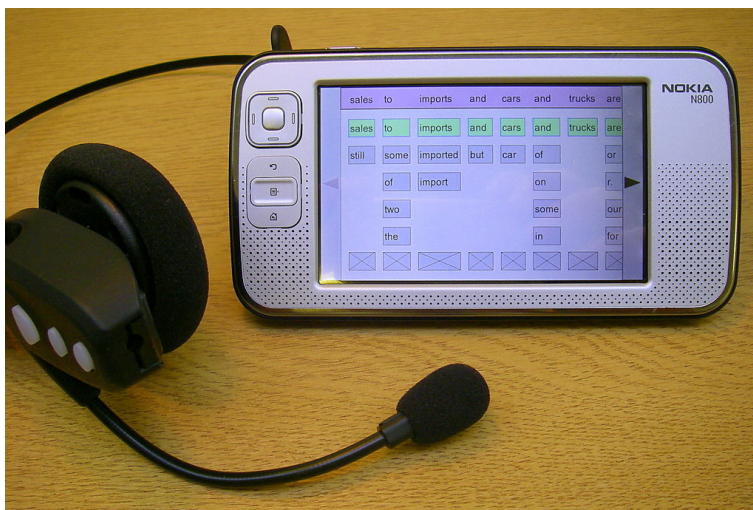
Figure 5.1: The Nokia N800 device and a Bluetooth headset. The Parakeet continuous speech recognition user interface is shown running on the device.
