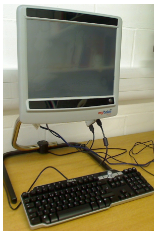
Figure 4.10: The MyTobii P10 gaze tracker used in the study. The tracking camera is built into the screen.
