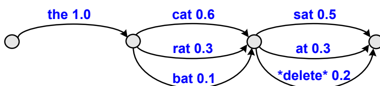
Figure A.5: An example word confusion network. The numbers on the edges represent posterior probabilities.
