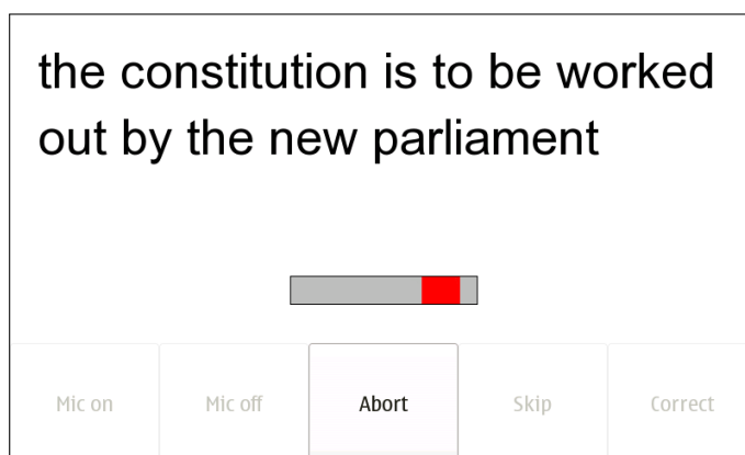
Figure 5.12: This screen presents the target sentences to the user. From left to right, the bottom buttons are used to: 1) turn the mic on, 2) turn the mic off, 3) abort a recognition, 4) skip to the next sentence, 5) move to the correction phase. If users needed a reminder of the sentence during correction, they could return to this screen by pressing the center button of the N800’s cursor pad.
