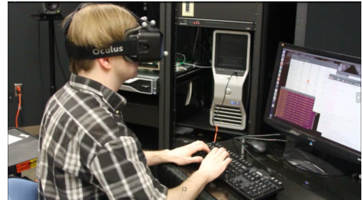
Figure 1. User typing on a keyboard while wearing an Oculus Rift HMD.
