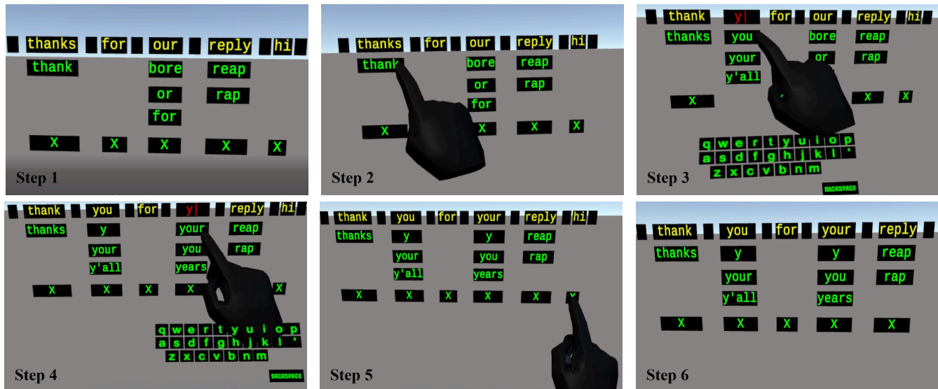
Fig. 2. Example of correcting a sentence using the speech interface. In step 1, the user has spoken “thank you for your reply”. The interface displays the most likely recognition result “thanks for our reply hi” in the top row. In step 2, the user selects the word alternative “thank” and it gets swapped with “thanks”. Next, the user needs to insert between the words “thank” and “for”. In step 3, the user taps on the blank space button appearing between these two words. The keyboard pops up and the user types the letter “y”. The user then selects the prefix completion “you”. In step 4, the user taps the word “our” in the top row. This opens the keyboard and after typing the letter “y”, the user selects the prefix completion “your”. In step 5, the user taps the button labeled X to delete the undesired word “hi”. Step 6 shows the text after all the corrections.
