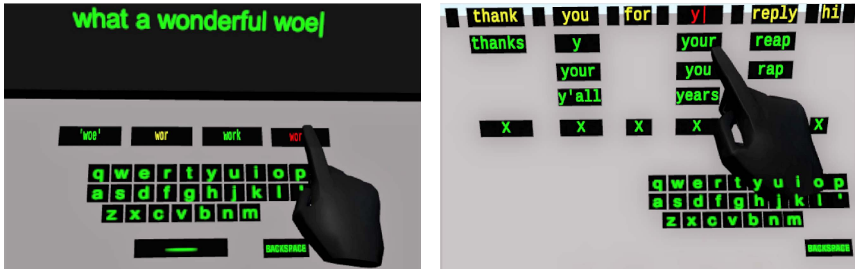
Fig. 1. We compare typing on a midair auto-correcting keyboard with word predictions (left) versus speaking a sentence and then correcting any speech recognition errors (right). Users correct errors by selecting word alternatives proposed by the speech recognizer or by typing on the virtual keyboard.
