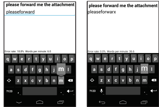
Figure 5. Google (left) and VelociTap interfaces (right) in Experiment 1. The user is tapping “m” and this key’s popup is being shown.
