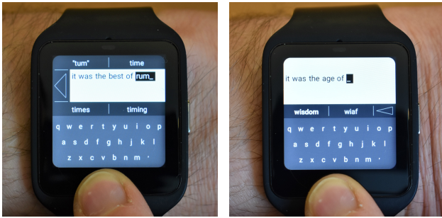
Figure 1: Entering text on the VelociWatch keyboard (left) and on a simpler version of the keyboard (right).
