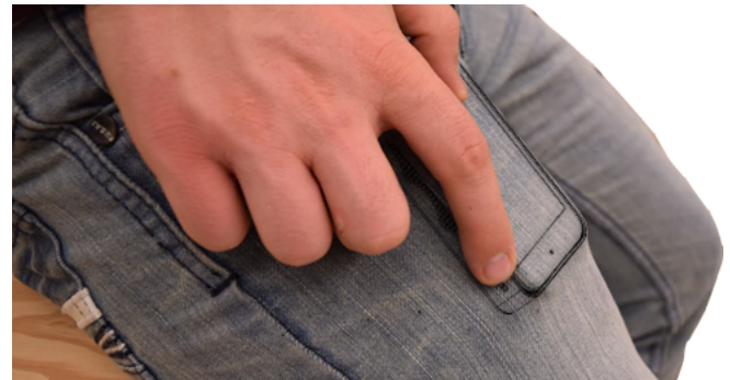
Figure 3: The Haptic Edge Display being used in-pocket for “pull” style haptic notifications.
