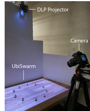
Fig. 5. Filming apparatus for the study: DLP projector producing a gray code pattern for localization, UbiSwarm as URI testbed, and camera for capturing video.
