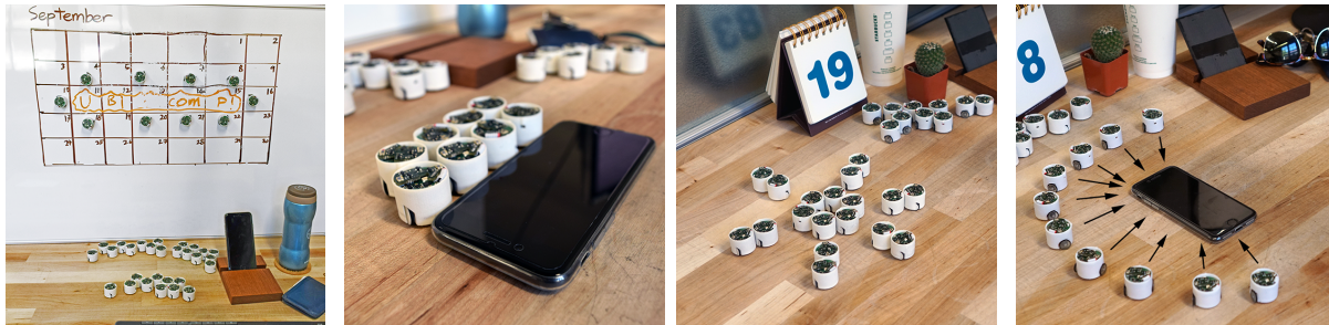
Fig. 1. URIs' mobility, manipulation and display demonstrated in situ. From left to right: UbiSwarm displaying calendar information on a vertical surface, UbiSwarm manipulating a mobile phone, UbiSwarm displaying iconic weather information, and UbiSwarm using abstract motion for a phone call notification.
