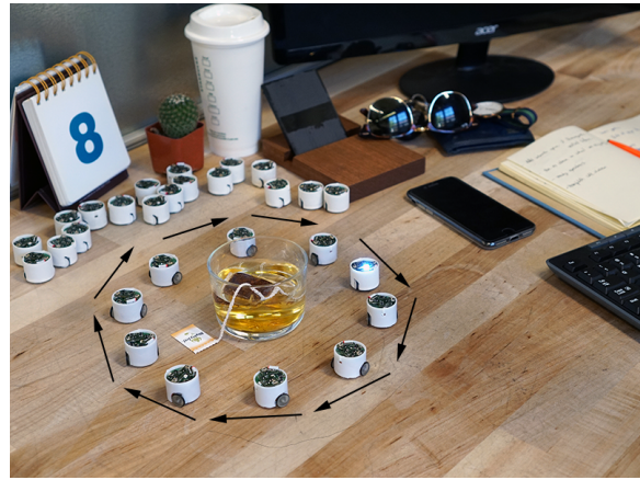
Fig. 10. Tea timer: UbiSwarm slowly and smoothly rotates around the tea acting as a timer and disperses when the tea is ready.
