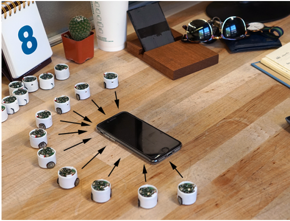
Fig. 9. Phone call notification: UbiSwarm rapidly and smoothly moves (rendezvous) toward a phone for notification of an urgent call.
