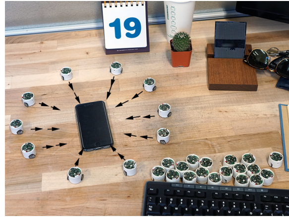
Fig. 12. Low battery notification: UbiSwarm slowly moves (rendezvous) toward a phone with synchronous jitter to signal low battery.
