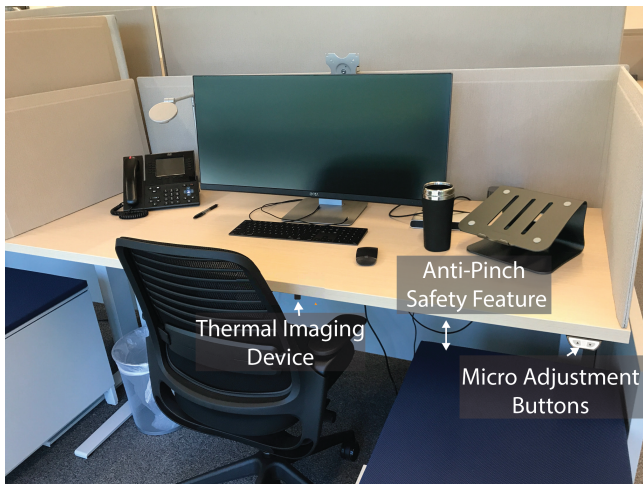
Figure 2: A commercial manual sit-stand desk was modified to change height automatically at preset intervals with an anti-pinch system for safety and a thermal camera to detect user presence and movement.
