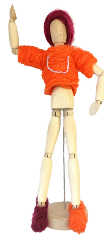
Figure 18: We change the shape of the cores to let the system make the hat, T-shirt, and shoes fit the doll's head, body, and feet. We combine the sleeves to the vest to form a T-shirt by felting the connection parts. We also decorate the T-shirt by felting the line on it. We use the puppet and the wearing on to show the possibility of quickly making the prototype of the textile.
