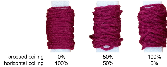
Figure 10: The figure demonstrates the cylinder results made with different crossed coiling ratios in the coiling way test.
