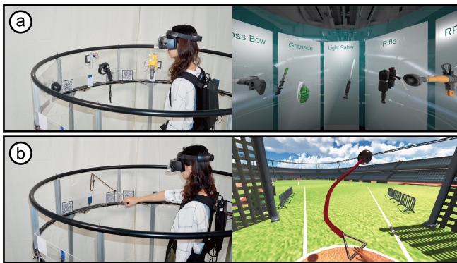
Figure 11. The finished experiences in our study2. (a) A battle game where the user can open up a menu to select weapons anytime. (b) A hammer throw game using the triangle as the grip and controlling the platform to simulate different weight.
