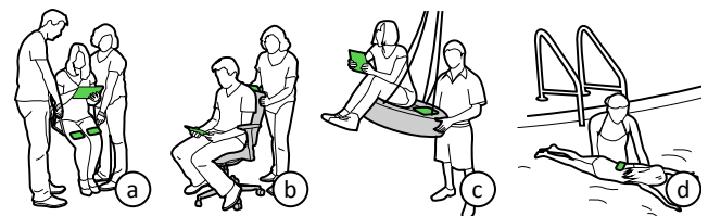
Figure 18: Haptic Turk configurations: (a) racing game based on two actuators, (b) chair and (c) swing allow for single-actuator use, and (d) in swimming pool.
