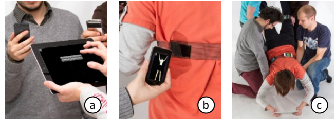
Figure 20: Setting up a haptic turk session via WiFi: (a) player starts a session, (b) joining actuator are assigned a position on the player's body, (c) play.
