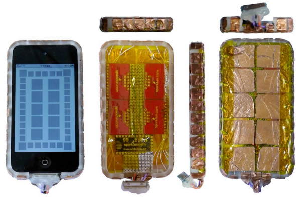
Figure 2: Photos of iRotateGrasp prototype, showing an iPod Touch, an Arduino board, 2 multiplexers, and 44 capacitive sensors in an iPhone 4S case.
