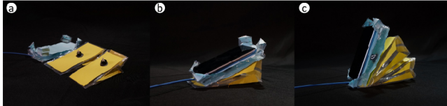
Figure 15: The smartphone holder made of PneuSeries in which the tilt angle can be programmed.
