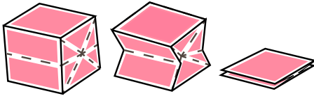
Figure 6: An illustration of our folding mechanism. The cubic inflatable folds along the gaps between the attached cardboard.
