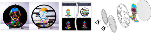
Figure 22: An anatomy diagram with user-dependent views, made with one mosaic, one mask, and two analyzers.
