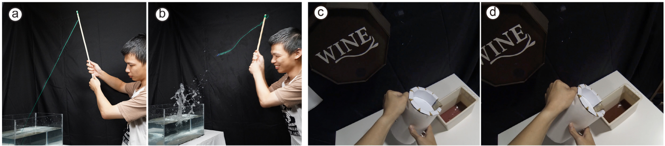
Figure 13: (a)The user is catching an imaginary fish with a fishing rod. The user feels the force from the fishing rod where its string is pulled by a motor and (b) sees the splash caused by the air compressor used in the catapult example. (c) The user pours imaginary wine into the kettle and sees (d) real wine being filled in the container through hidden tubing underneath it that is connected to a wine pump.
