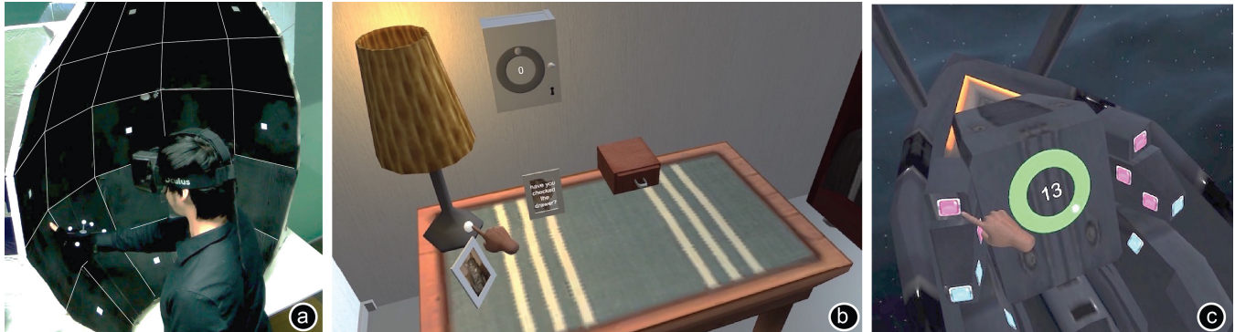
Figure 1. (a) Our hemispherical prop is an example of a Sparse Haptic Proxy . It simulates both, (b) a room and (c) a cockpit scene to provide physical touch feedback during interaction. (White lines on the prop added for visibility on the black background).
